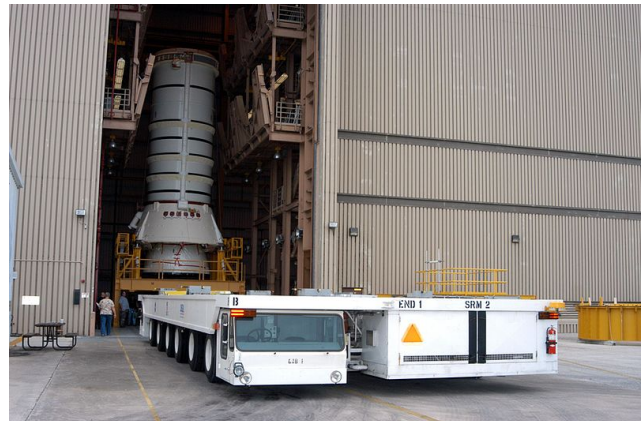
Solid Rocket Motor transporter vehicle manufactured by Kamag
